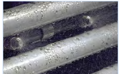
The UV3 reproduces the damaging effects of thermal shock and mechanical erosion
