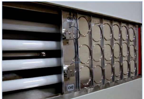
The Solar Eye's UV sensors are located in the specimen mounting plane
